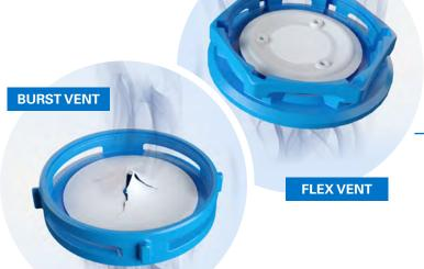
In the case of rapid pressure and heat buildup, the second stage helps maintain internal enclosure pressures by allowing gases to escape by either bypassing the membrane with the umbrella flex or bursting the membrane.
