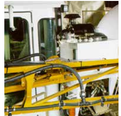
The FRG Air Cleaner on this Tyler Ag Sprayer eliminates 99.99% of the dirt from the engine airstream, while providing up to 945 cfm airflow to the engine.
