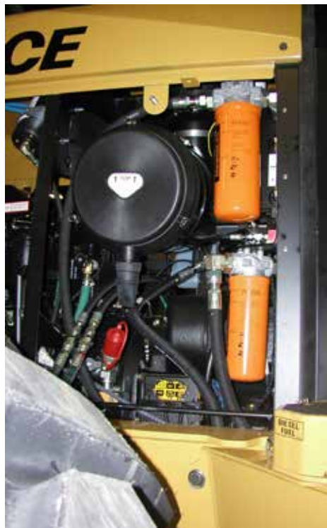
The two-stage FRG Air Cleaner in operation on a Prentice 490 Skidder.
