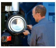
When servicing the EBB, make sure to replace the cover gasket when changing filters.
