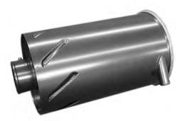
The FLB - Louvered Body Air Cleaner is a two-stage air cleaner with scavenge exhaust system and Axial Seal Sealing Technology. Body diameters in 6", 8", 10" and 12". Handles airflows of 3-17 m<sup>3</sup>/min. Sustained temperature tolerance: to 82°C.
