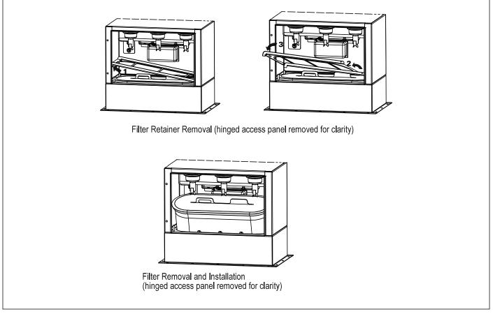
Filter Removal and Installation for CPV-1 Collector
