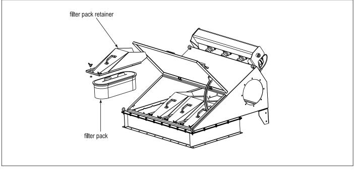
Filter Removal and Installation
