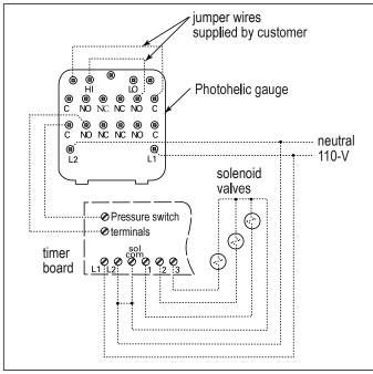
Photohelic Gauge Wiring Diagram
