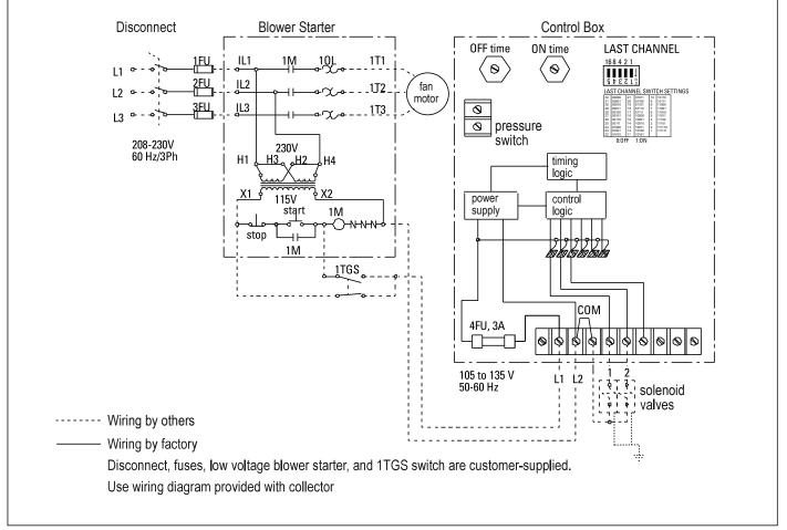
Solid-State Timer Typical Wiring Diagram
