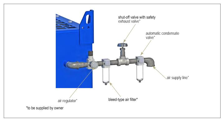
Compressed Air and Component Installation
