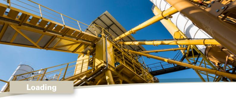
From the grinding mills, the cement is conveyed to silos where it awaits shipment, depending on type and strength class. From there it is mainly loaded in bulk form from terminals onto rail or road vehicles as well as onto ships.
