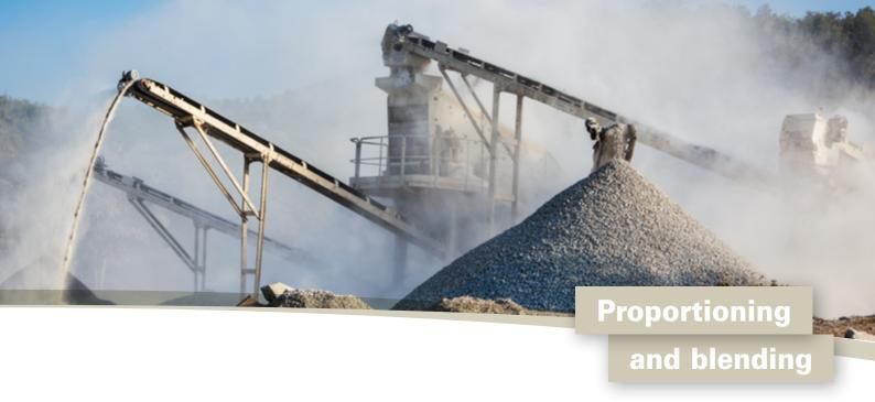
The crushed material is transported into the raw material storage of the cement plant by conveyor-belts, cableways or railways and in exceptional cases with trucks. Once there, it is stored in blending beds and homogenised.
