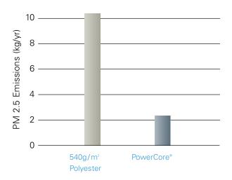
These flat sheet results are based on independent lab tests using ASTM D6830-02 per EPA PM 2.5 performance verification. Annual emissions calculated assuming 24,466 m²/h airflow rate, 265 working days per year, and two shifts per day. Field measurements may vary due to differences in dust contaminant and sensitivity of measurement equipment.
