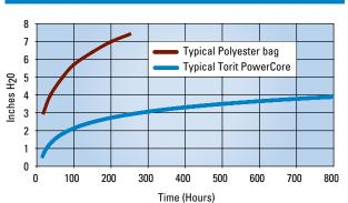
The results from accelerated lab and field tests show that Torit PowerCore can provide lower pressure drop in baghouse applications.
