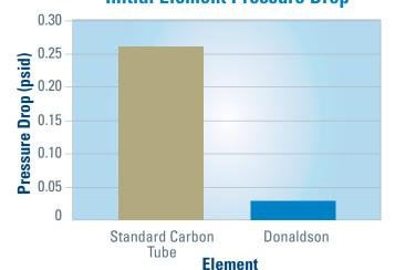
Donaldson's GSL N element reduces the differential pressure by  $8\mbox{\scriptsize X}.$
