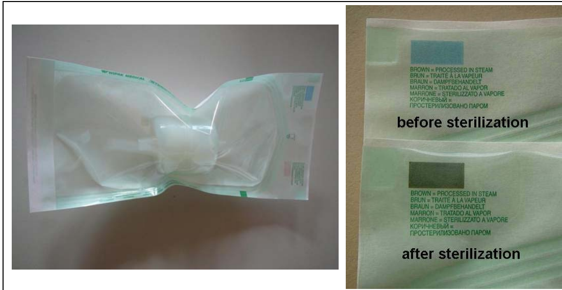
Figure 19: Capsule filter in special sterilization bag; the indicator on the bag changes color when in contact with steam
